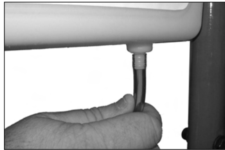
Figure 3 - Attach suction tube to barb fitting
